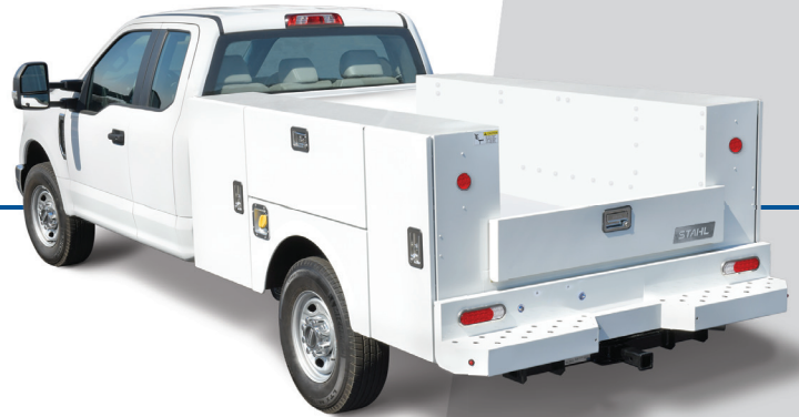
Body pictured with optional Recessed Punched Bumper with surface-mounted LED 3-in-1 Light Kit and Aluminum Fuel Fill
